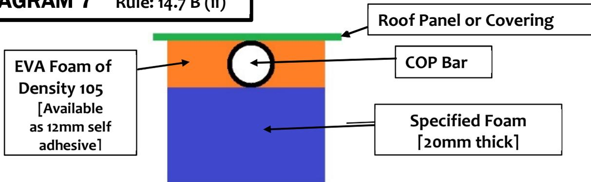
A suggested way of providing protection when a COP bar is directly above a rider
